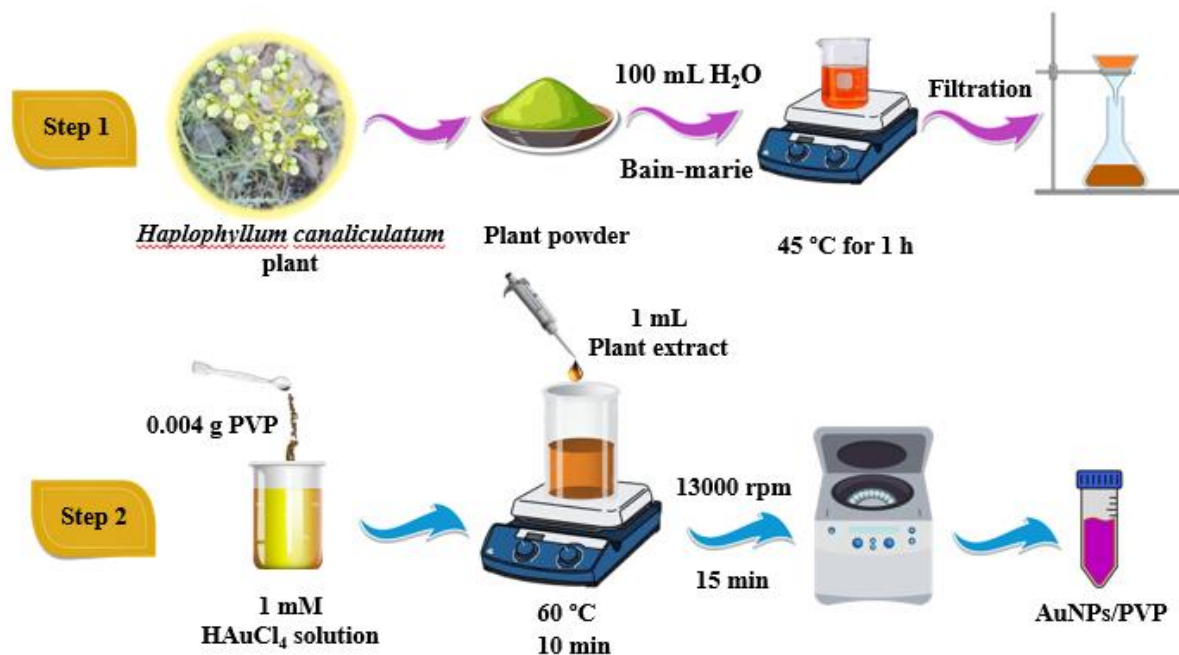
Figure 1. Schematic illustration of the synthetic strategy of AuNPs.
